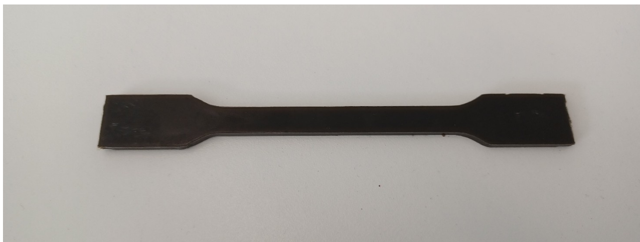
Figure 5. Injection-moulded tensile test specimen made from recycled netting material.
