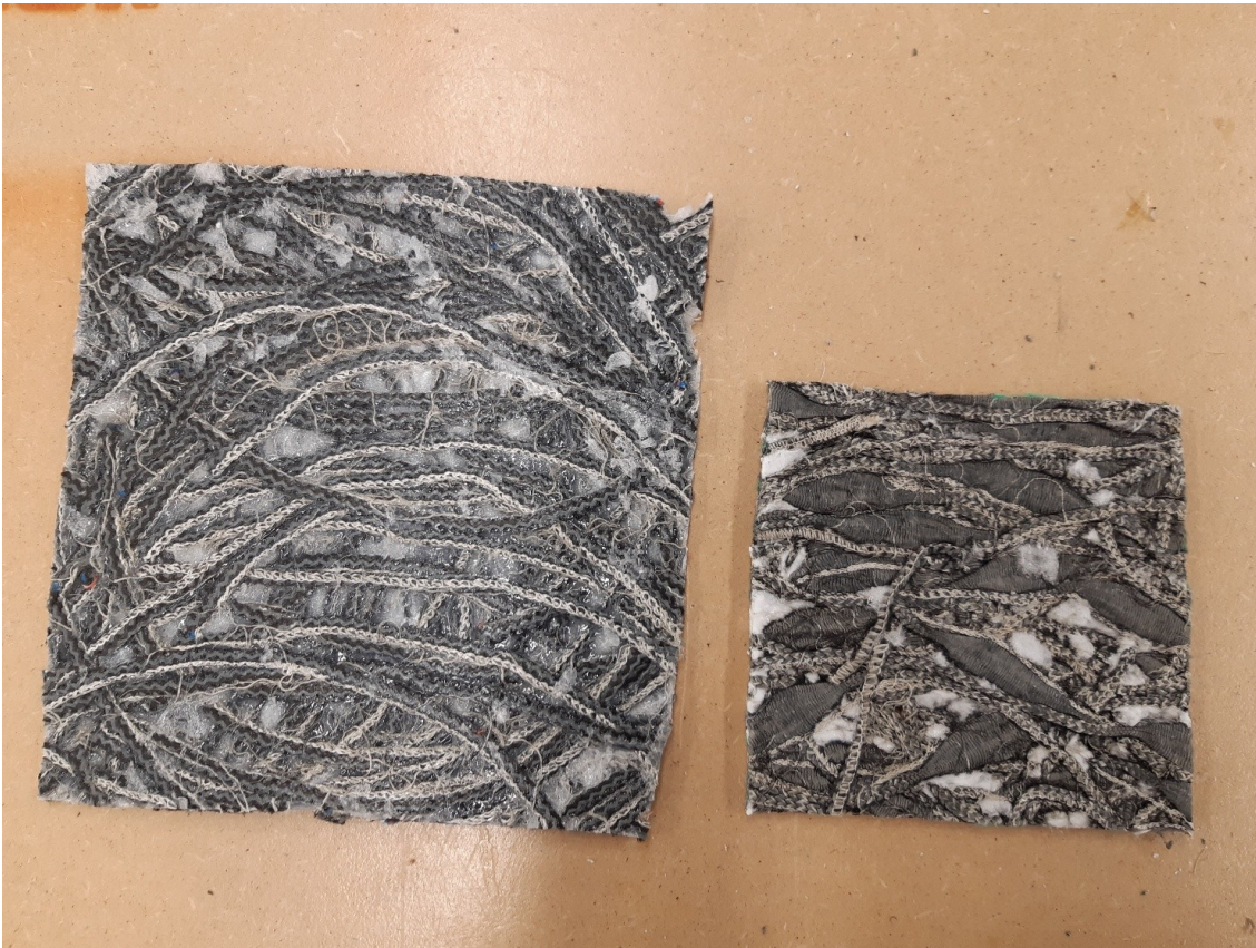
Figure 7. On the left, a plate pressed from the lower float lines; on the right, a plate pressed from the upper float lines.
