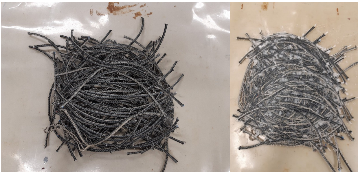
Figure 6. On the left, unpressed lower float lines; on the right, a compression-moulded plate made from lower float line material.
